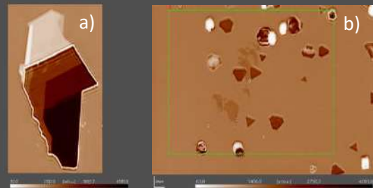
Figure 16. Ellipsometric contrast micrographs of hex-BN Multilayer (a) and 2D antimony telluride ( \text{Sb}_2\text{Te}_3 ) nanoplates (b).
