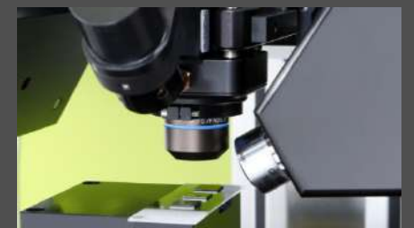
Figure 15. Integration of a Micro Raman into the setup of the nanofilm_ep4.
