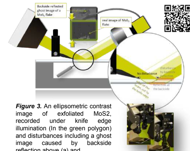
Figure 2. EP4 with illumination arm on the left and Analyzer arm with the optical system at the right. The sample can be placed onto a motorized xy-table.
