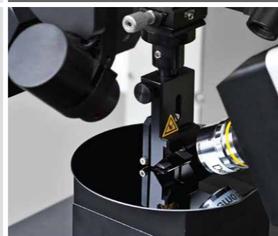
EP4 beam cutter – a nondestructive way to eliminate backside reflection
