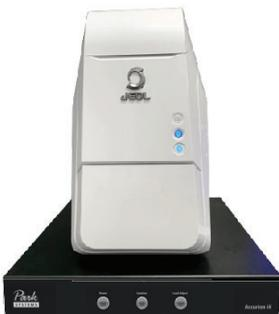
▪ Scanning Electron Microscope on Accurion i4 Medium (JEOL Neoscope)
